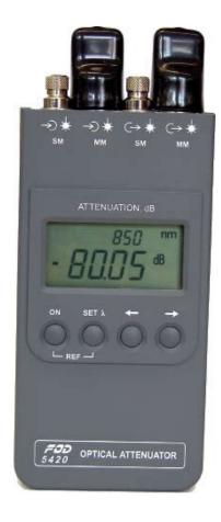
The FOD 5418, 5419, 5420 Variable Optical Attenuators are designed to simulate optical attenuation when checking the optical margins of newly installed telecommunication equipment. The device is suitable for singlemode application at 1310 and 1550 nm (FOD 5418), multimode application at 850 and 1300 nm (FOD 5419), or both singlemode and multimode application at 850, 1300, 1310 and 1550 nm (FOD 5420). They allow variable attenuation settings in range from 0 to 80 dB with resolution 0.05 dB.
