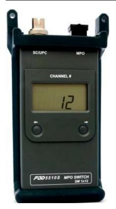
The FOD 5510 Series Fiber Optic Switches are a compact, robust, battery operated 1X12 switch designed specifically for use with OTDRs and Optical Loss Testers for certifying, testing and troubleshooting MPO terminated cables and harnesses. Whether used in manual mode with pushbutton controls, or automated with USB Windows® or Linux® based remote control drivers, the FOD5510 Series brings multi-fiber testing to a new level.
